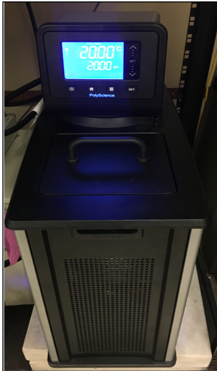
Figure 3: Circulating water bath
