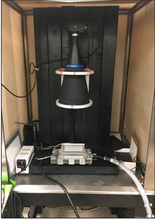
Figure 2: Photograph of behavioral assay setup including telecentric lens and digital camera.
